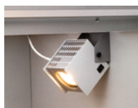
FX-CMB Accessory directional light source for gonio-apparent coatings
